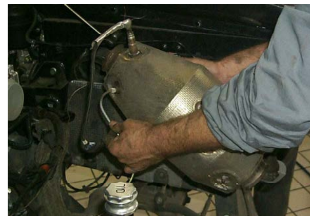
Fig. 8 Right catalytic converter removal
