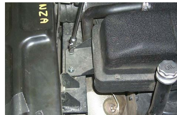
Fig. 3 Air filter support fastening screws removal
