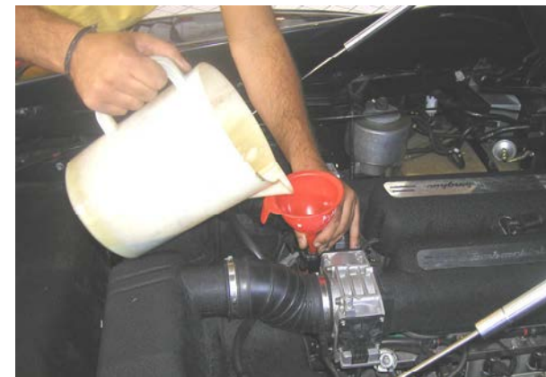
Fig. 3 Gearbox and rear differential oil filling
