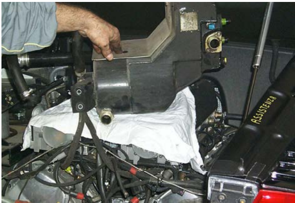
Fig. 11 Engine oil tank positioning
