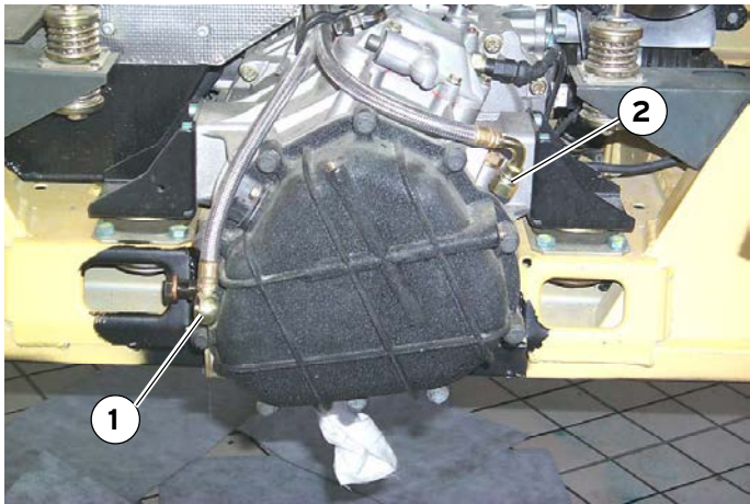
Fig. 15 Radiator gearbox oil pipes
