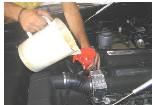
Fig. 3 Topping up the gearbox and rear differential oil
