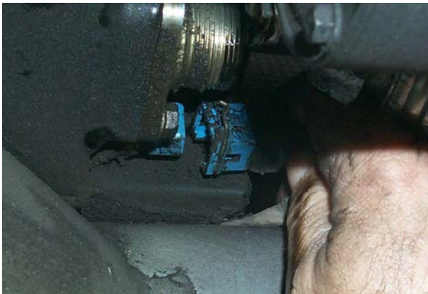
Fig. 9 Engine oil temperature sensor disconnection
