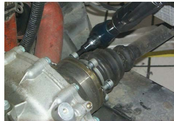
Fig. 14 Axle shafts disconnection
