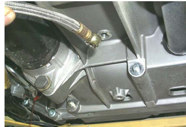
Fig. 11- Clutch hose disconnection
