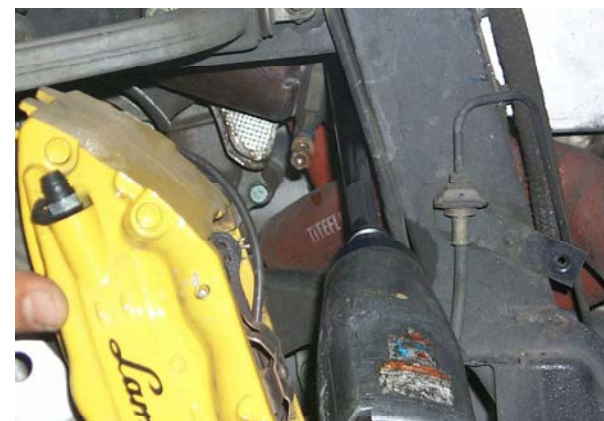
Fig. 7 Catalytic converter fastening clip loosening
