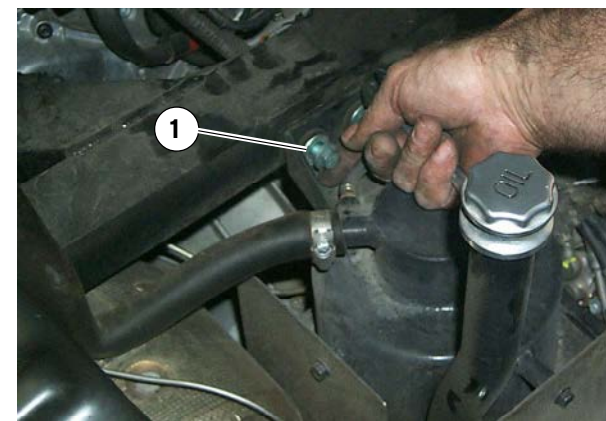
Fig. 5 Engine oil tank fastening screws removal
