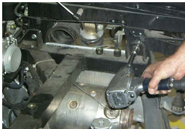
Fig. 6 Central cross member removal
