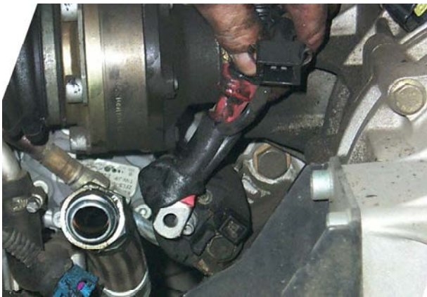
Fig. 16 Starter cables disconnection
