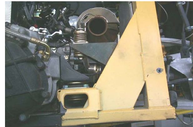
Fig. 19 Loosen the engine fastening bolts
