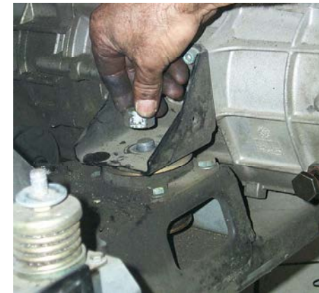
Fig. 17 Gear supports screws removal
