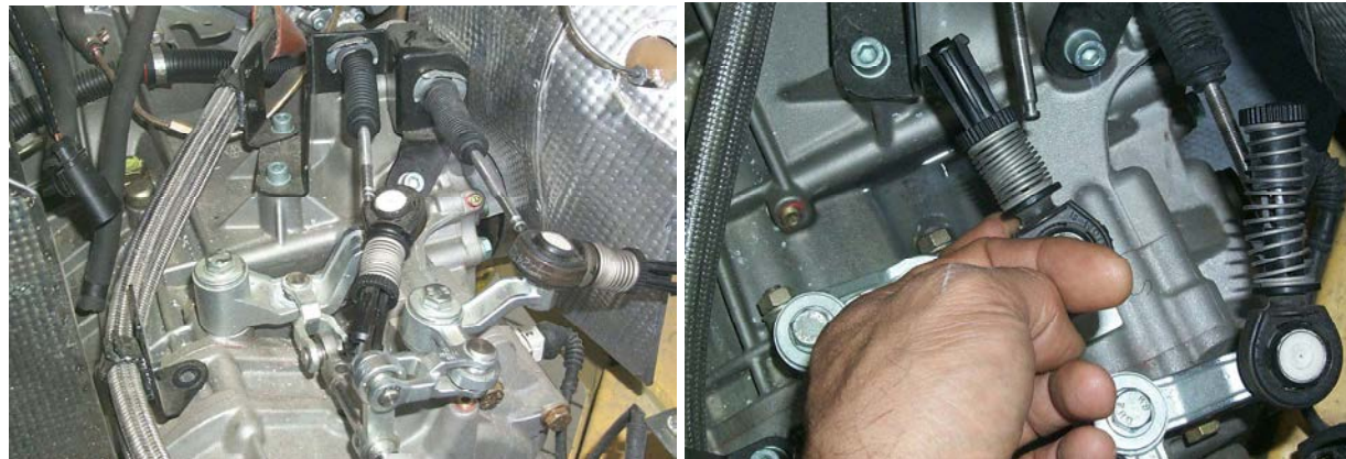
Fig. 12 - Selector cables removal
