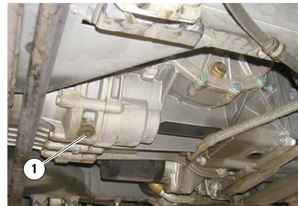
Fig. 1 Gearbox and rear differential oil draining plug
