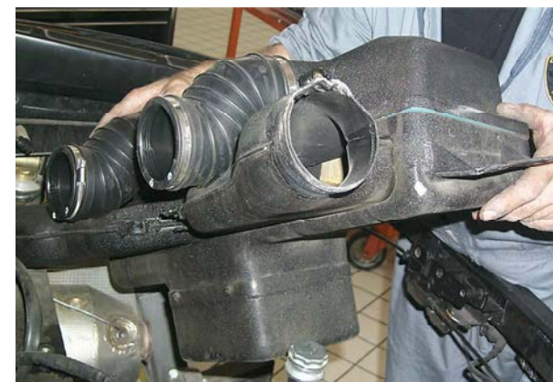
Fig. 4 Air filter support removal
