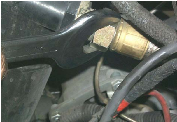
Fig. 10 Engine oil tank input and output pipes disconnection
