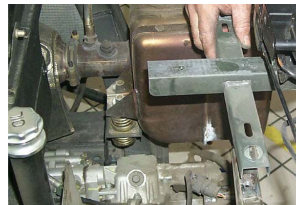
Fig. 1 Rear central cross member removal
